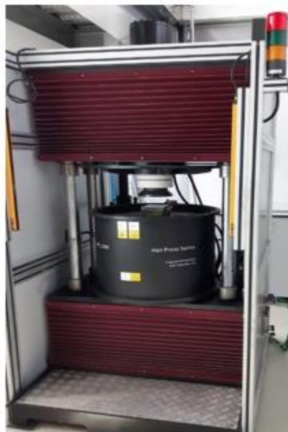
Figure 1. Hot pressing device for composite production.
